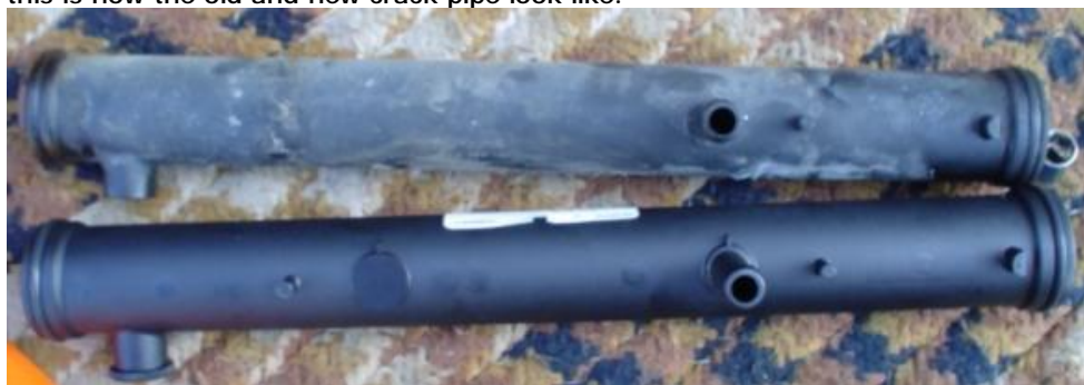
this is how the old and new crack pipe look like.
