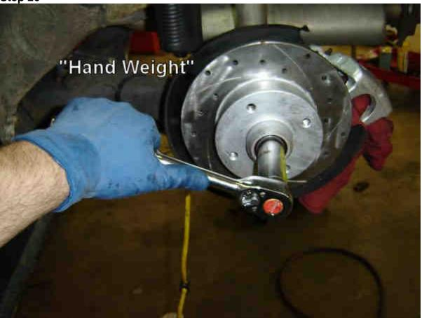
Lightly lube the spindle with the same grease you used for the bearings. Install the rotor, with its new races, and bearings onto the spindle. Install the washer and nut and then hand tighten the nut as you spin the rotor backwards.
