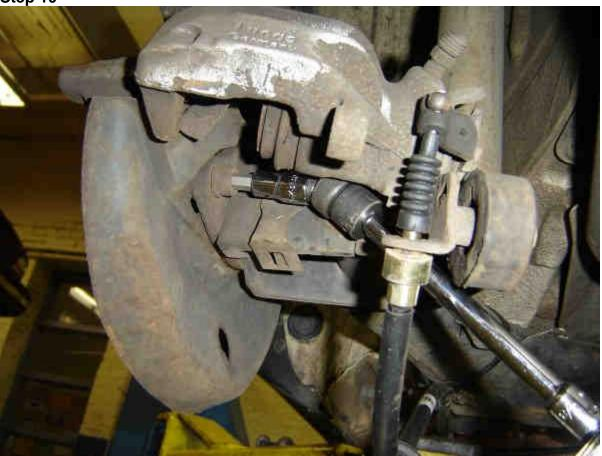
Take the 8mm allen socket and remove the two caliper carrier (pad carrier) bolts. These are tight, and sometimes, break. Use a top quality brand 8mm allen socket. Forget the wimpy "T" handle wrench. Make sure the 8mm socket is fully seated into the bolt. Tap it with a hammer, or use a small screwdriver to clean the allen bolt out. You'll have to use a long handle 3/8 drive ratchet and a few extensions and that universal swivel to get to them.
