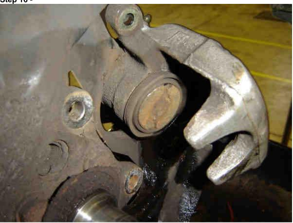
Once its pushed back into its bore, it should look something like this. Use the brake clean to clean off the caliper, and dust shield.
