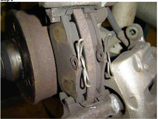
Once you get the caliper bolts off. Move the caliper off its mounts, and swing it to the rear. Try not to let it hang by the brake hose. Use a coat hanger if you have to. Slide the pads out. The metal shims can go in the trash if you ask me.
