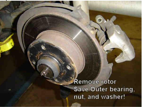
Save and clean the nut and washer. Pull the rotor off the hub. Check out the bearings and see how they fit with the spindle.
