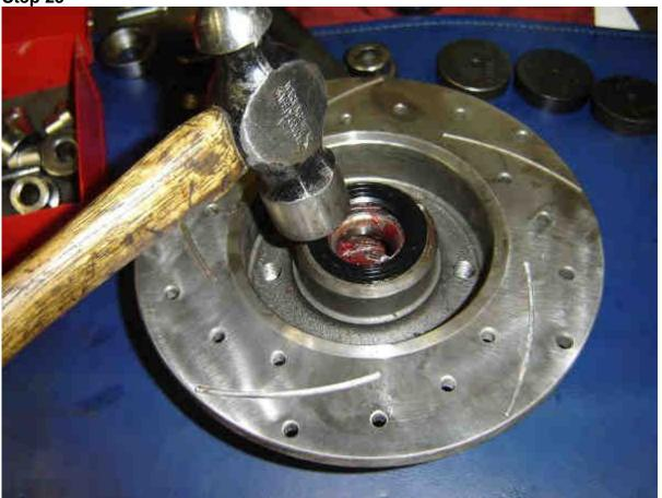
Lube the bearing (how to here - pdf), and then install it (again check to make sure its going in the right way!!). Tap the grease seal into place.
