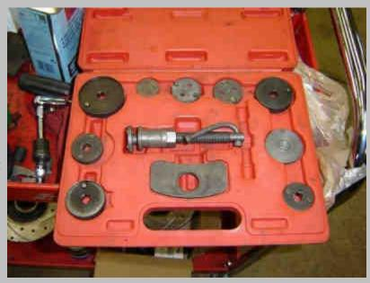
Caliper Retractor Tool (set) - A must have for this job (for pushing back the caliper) (Shown to right)
