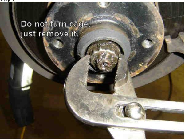
Once the cotter pin is out. Pull the nut cage off. Pull it off "towards" you.
