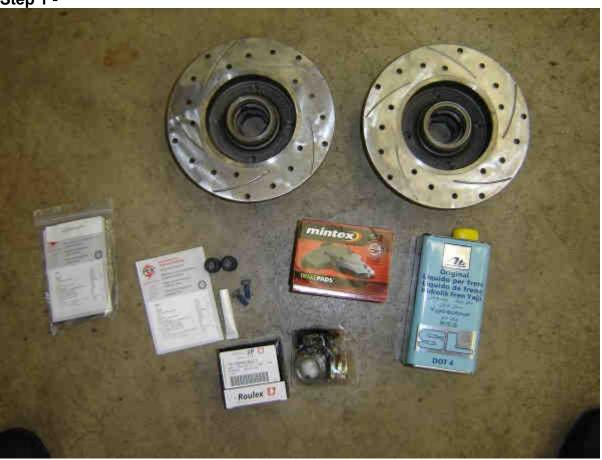
Start with some quality parts. I got a good deal on the Bahn Brenner rotors, such a good deal I could not pass them up. Slotted and cross drilled rotors look sharp and stop the car nice and quick. I also got a full bearing kit, ATE DOT 4 Brake Fluid, Caliper boots, Caliper slide bolts, and Mintex Red Box pads. Honestly the rotors are total over kill for me and my drive to work, but like I said, they do look sharp.
