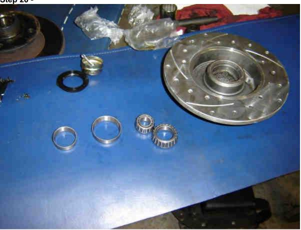
Here we see the cotter pin, dist cap, dust seal, outer race, (smaller) inner race (bigger), outer bearing (smaller), and inner race (bigger), and the rotor.
