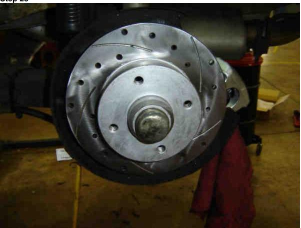
Install the dust cap. Give the rotor a spin and make sure the cap is not hitting any of the cotter pins. Take a clean rag and some brake clean and wipe off any grease on the rotor faces. The silver is not anti-seize compound, but rather silver caliper paint. This keeps the rotor hat from rusting and looking like crap after a year.
