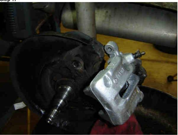
I hit the caliper with some silver caliper brush on paint, and painted the dust shield with black paint. Looks a little better. Let it dry while we go onto the next step.
