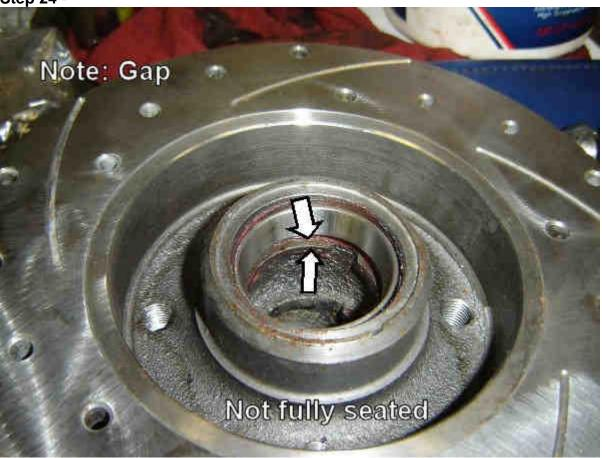
Make sure you don't have a gap here, the seal driver and hammer will change sounds once the race is fully bottomed out into the rotor race bore.
