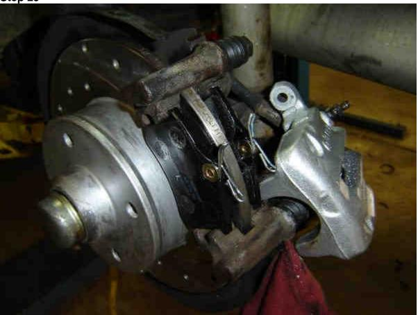
Slide in the new pads. If needed peel off the noise sticker, or add brake antisqueal compound to the pads. I threw the factory shims in the trash. Really...
