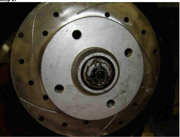
Next install the cage nut and cotter pin. The cage nut can line up pretty close with the holes in the spindle. If not, a slight, very slight over torque is ok. Fold over the cotter pin's legs as shown.
