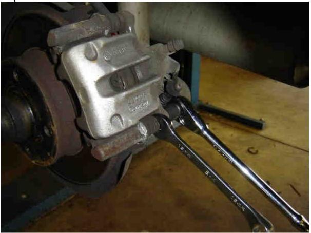
Use the 15mm wrench and the 13mm socket. Hold the flats on the caliper slides with the 15mm wrench. You might need a thin wrench to do this, turn the 13mm socket counter clockwise to loosen it. Do this for both the upper and lower (shown) caliper bolts.
