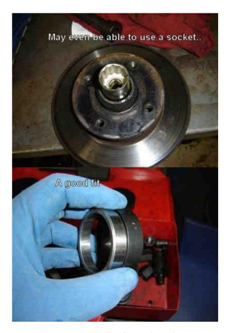
Make 100% sure your driver is the right size. You do not want it to get stuck in the rotor, or be too small and smash into the bearing race face.
