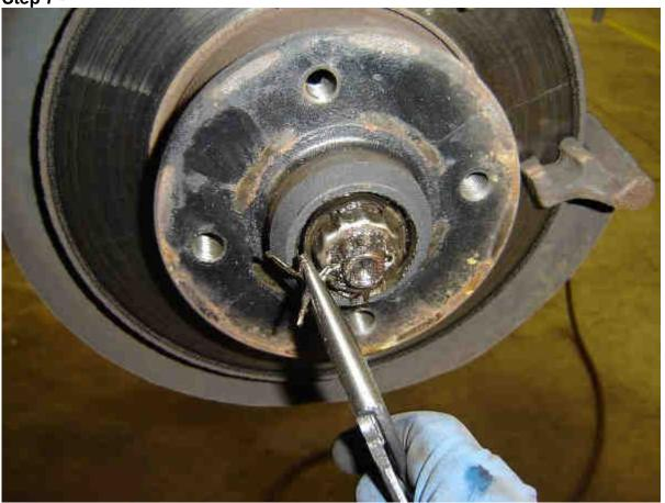
Using the needle nose pliers, pry out the old cotter pin. **NEVER REUSE A COTTER PIN! THROW IT THE HELL OUT! DON'T USE A NAIL OR A PAPERCLIP IN ITS PLACE!! IT HOLDS THE WHEEL ONTO THE HUB!!!**
