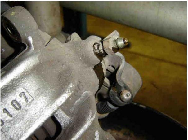
Go under the hood and open the brake fluid reservoir. Top off the fluid, and leave the cap loose. Back to the caliper, remove the rubber cap on the brake bleeder - using the 11mm wrench, open the bleed screw until some brake fluid runs out.
