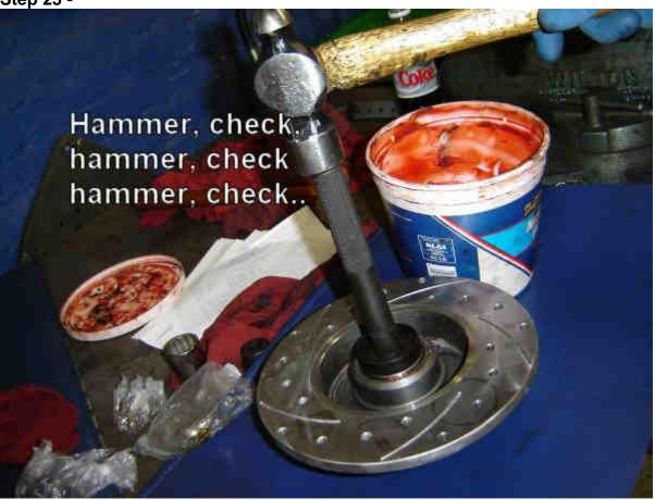
Hammer, and check to make sure the race is being driven in straight. If it starts to get all crooked STOP and tap it flat.. If it gets real crooked, you can use a punch to hammer it back out from the backside.
