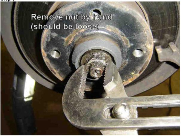
Once the cage is off. Turn the nut to remove it. It should be loose (THIS IS NORMAL).
