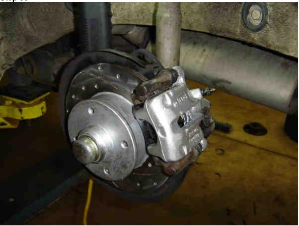
Put the wheel on, spin the wheel by hand, check for bearing end play.
