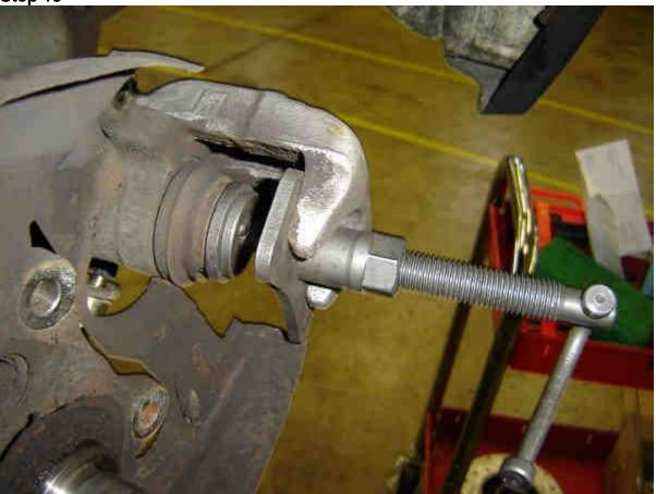
Place a pan under the caliper to catch brake fluid from the bleed screw. This will push out the old fluid into a pan, rather than back up into the brake system.
