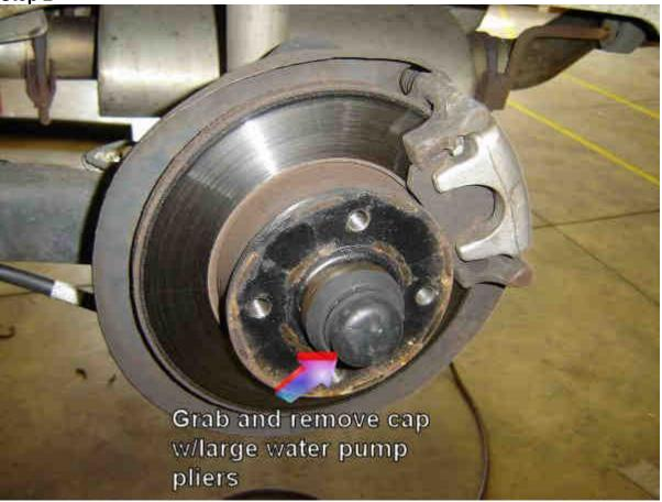
Once you get the car up in the air, and <u>remove the wheel</u>. Make sure the parking brake is off. Use the large "channel lock" pliers and pull the cap off. Try not to crush it. If its stuck, tap it gently with a rubber hammer.
