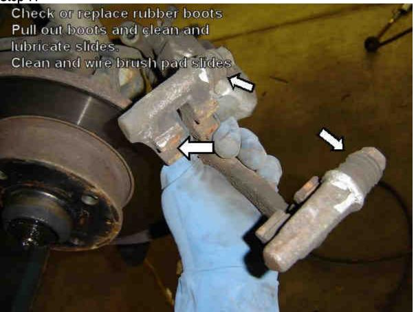
Pull the pad/caliper carrier off the axle. Be careful not to have the rotor fall off (cause it can!). Clean the points shown, check the boots, lube the caliper slides. Clean the pad slides with a wire brush or 600 grit sand paper. VW says to always replace the caliper slide bolts, I say - eh.. use more blue Locktite. I DID get "the kit" this time. It comes with new boots, grease, and of course the new bolts with the blue Locktite on them.
