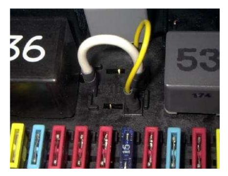
This is an easy mod. You must realize, though, that all the current of the lights must pass thru the jumper. So you must use a decent size wire. I used a 12ga jumper for the fogs. But since I have my headlights relayed, I only needed a small wire for the lowbeam jumper. Without relays, I would have made that jumper larger also. The problem with that is those pins are small and it would be difficult to connect 12ga wire to them.
