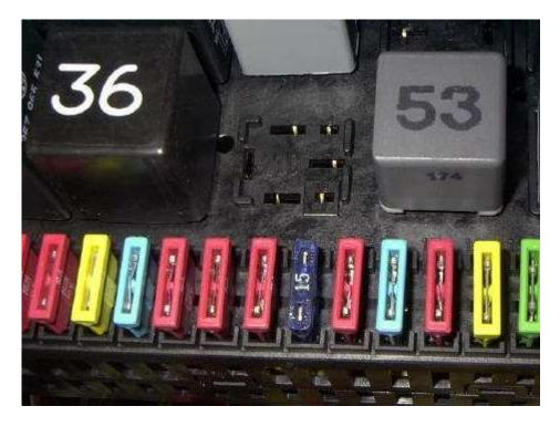
If you jumper the vertical slot on the left to the slot directly to the right of it, your fogs will stay on when you switch the lights to high beam. Like this.
