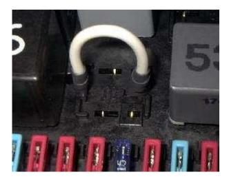
If you jumper the two small slots at the top and bottom right corners, your low beams will stay on when you switch to high for maximum light. Like this.
