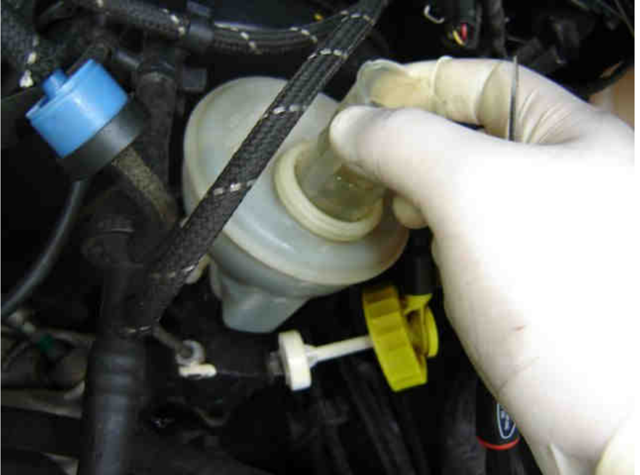
Pulling out the master cylinder filter.
