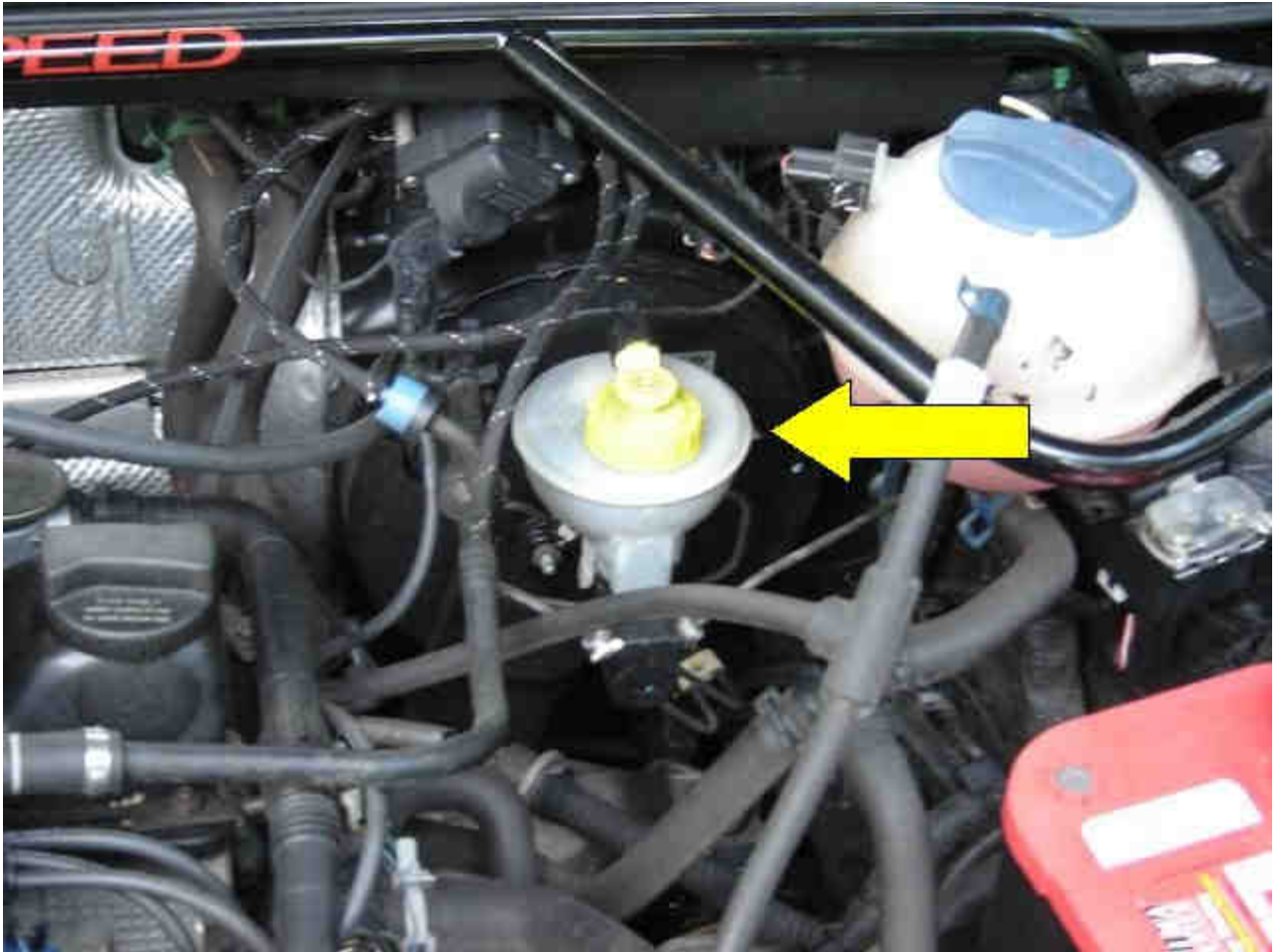
The master cylinder has the yellow cover.
