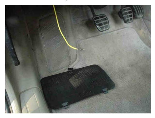
We now need to remove the panel that's on top of the pedals (in between the knee bar and the body of the car, under the fuse box, precise enough?).
