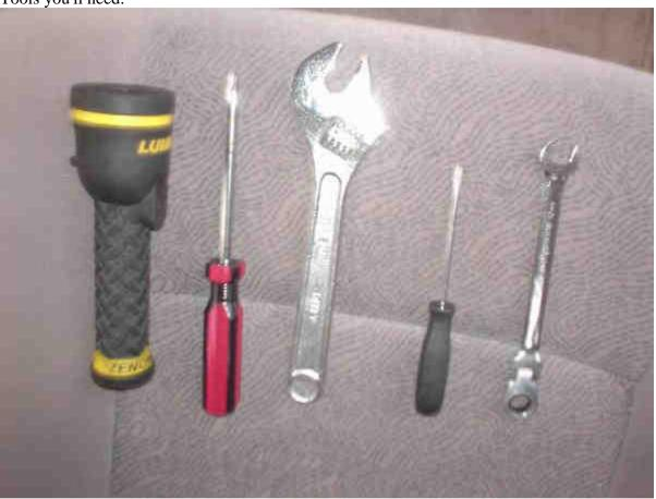
Flash light (as small as possible), philips head screw driver (a #2, not the small small, neither the small, but the "medium one" otherwise you'll strip bolts' heads like crazy), an ajustable key (whatever that thing is called), a small flat head screw driver and a 10 mm key with a ratchet at the end of it.
