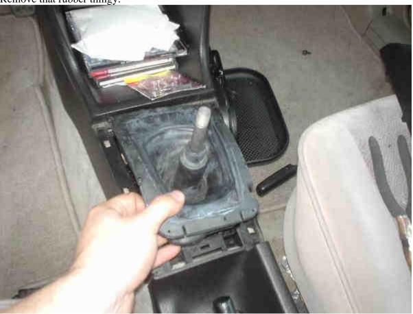
Take the 10 mm key/wrench and remove the 2 plastic nuts in between the shifter and the arm brake. I wouldn't use a key here because you might strip the nuts.
