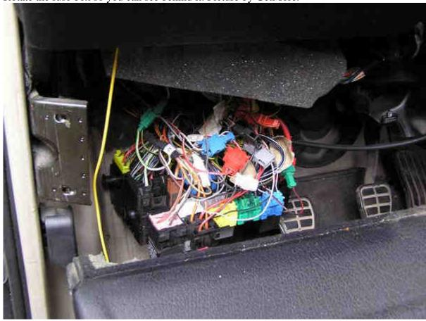
We're looking for the P6 connector. It's blue and removed on this picture. Picture from GetMore.
