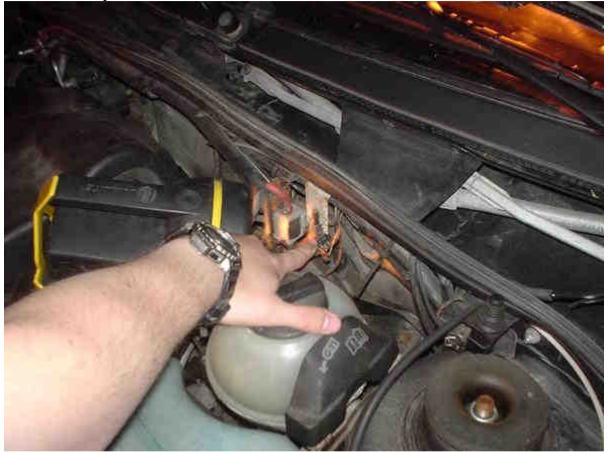
As you see the relay is besides the N75 on the firewall, behind the coolant reservoir.
